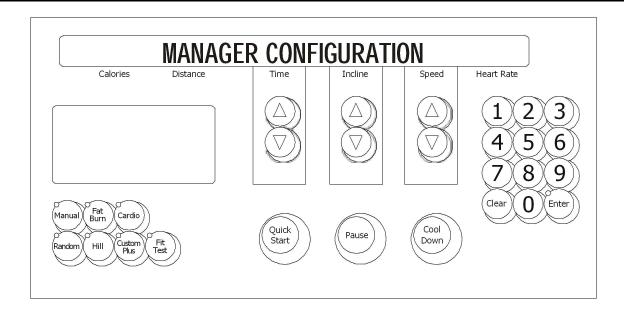
The information will automatically scroll every 3 seconds or using the 'TIME UP' or 'TIME DOWN' arrow keys will allow you to scroll through the configuration items.
